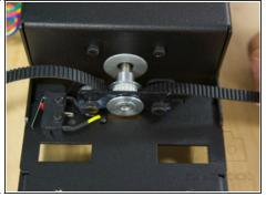
Run a GT2 belt over the 624 bearing, under the GT2 pulley, and back up over the other 624 bearing. The teeth of the belt should be facing up and aligned with the grooves of the GT2 pulley.
