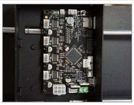
Attach the Printrboard to the bottom of the base with M3 6MM screws (x4). Note that the SD card port slot and micro-USB port are facing out, aligned with the holes in the base.
